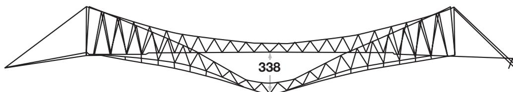
New suspension with triangulated hangers and lateral stabilizing cables.
